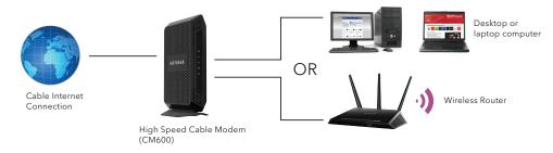
Connect the CM600 High Speed Cable Modern directly to your computer or wireless router for connecting to other wireless devices.
